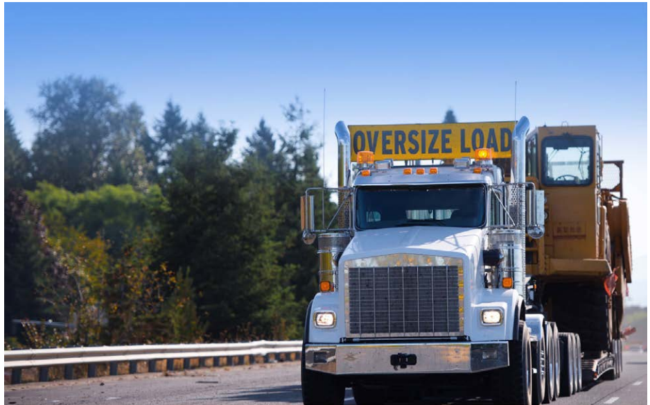
A tractor-trailer moving an oversized load on a state highway requires an OS/OW permit and routing.
