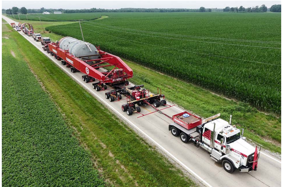
Illinois DOT used the Illinois Transportation Automated Permits (ITAP) system to manage the routing and bridge analysis for an oversized load, weighing nearly 900,000 lbs., moving from Tulsa, Oklahoma to Robinson, Illinois.
